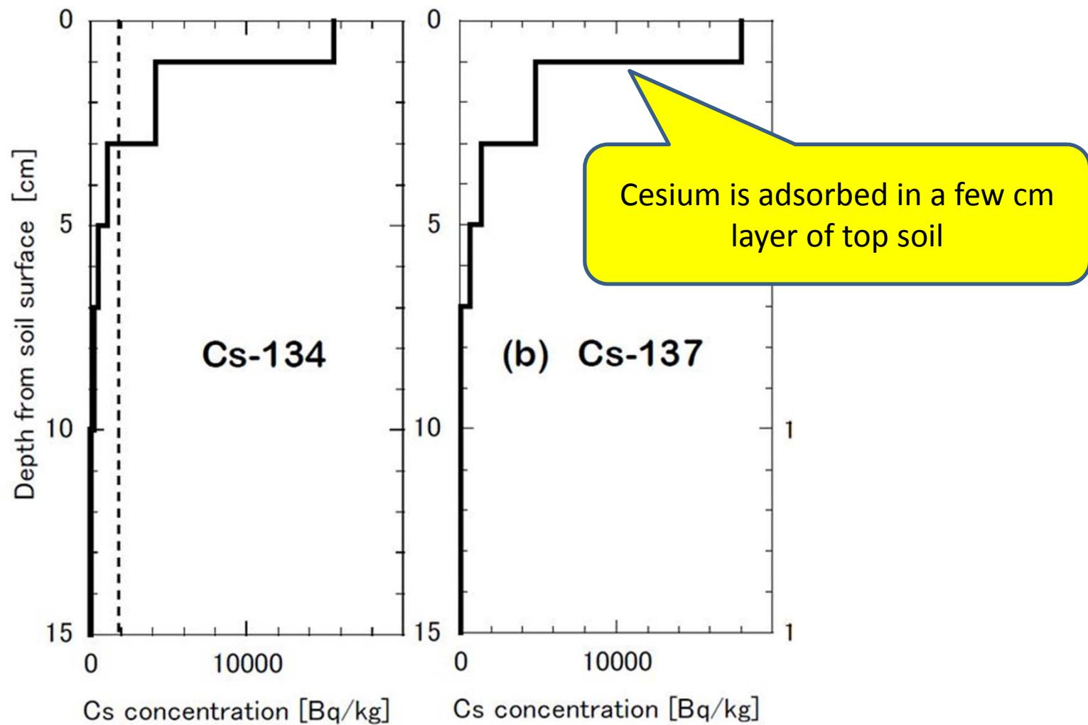
Shiozawa, et.al: Vertical Concentration Profiles of Radioactive Cesium and Convective Velocity in Soil in a Paddy Field in Fukushima, RADIOISOTOPES, 60, 323-328 (2011)
