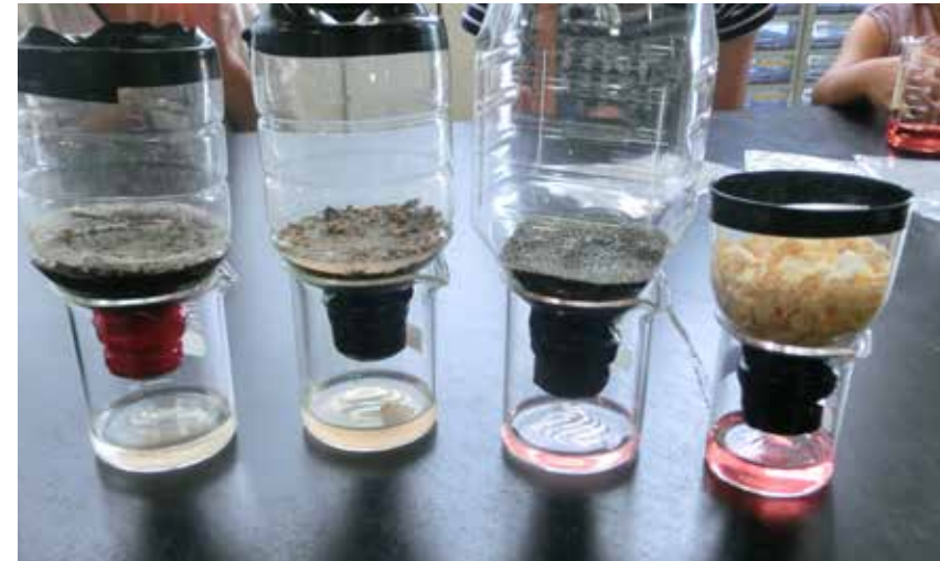
Adsorption experiment using plastic bottles (from left: field soil, mountain soil, sea sand, sawdust)
