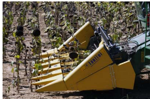
Figure 5. General combine modified with a picker header Figure 6. Sunflower picker header by produced fantini company http://www.fantiniworld.com/public/images/4062.jpg
