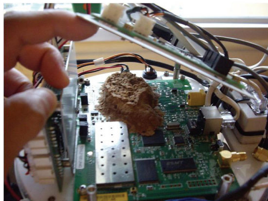
Fig. 4. Insect nest built on CPU board of Field Server
