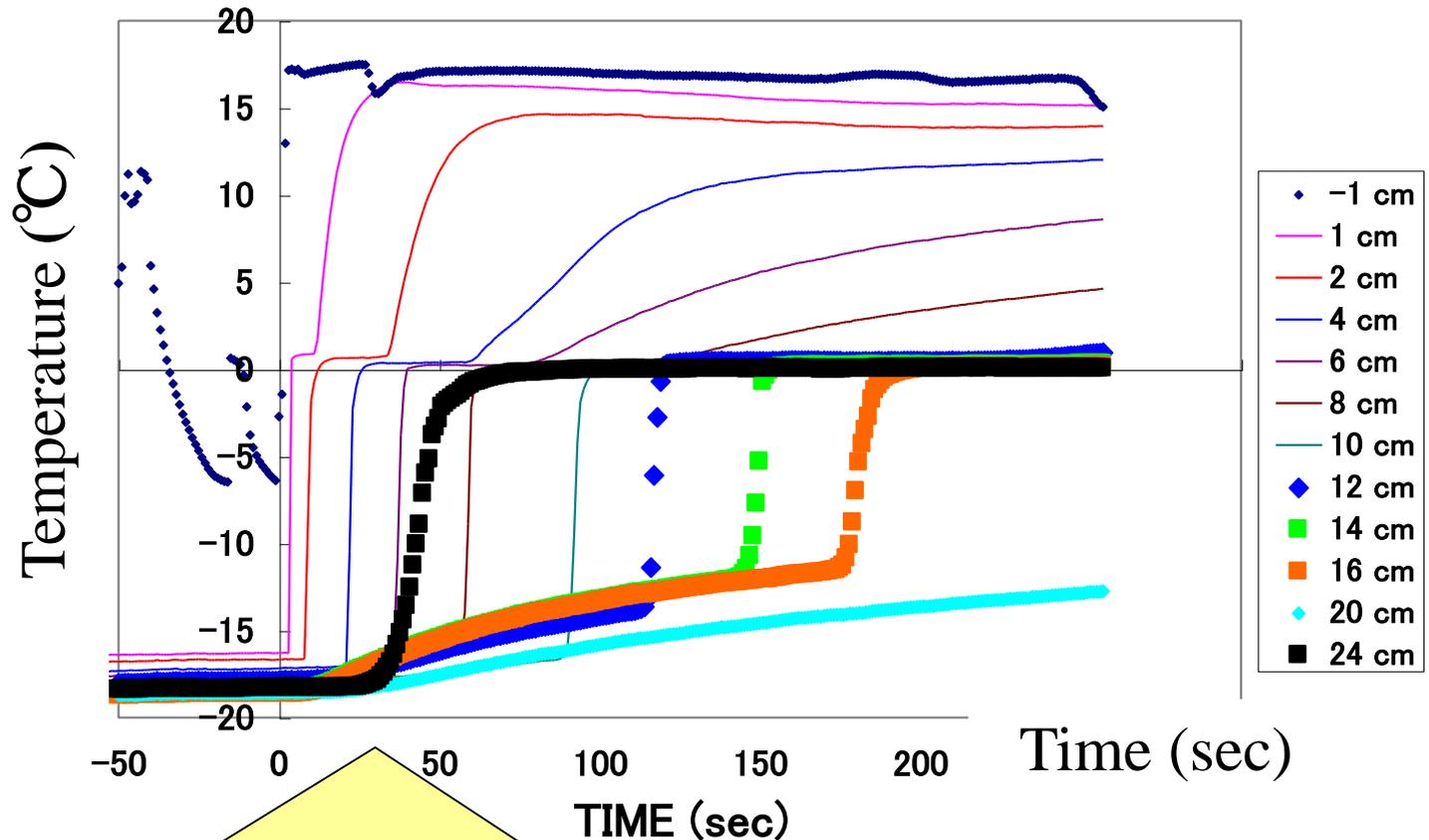
**Temperature at 24 cm increases faster than at 10-20 cm, and temperatures at 14 cm and 16cm increase slowly before abruptly increase.**
