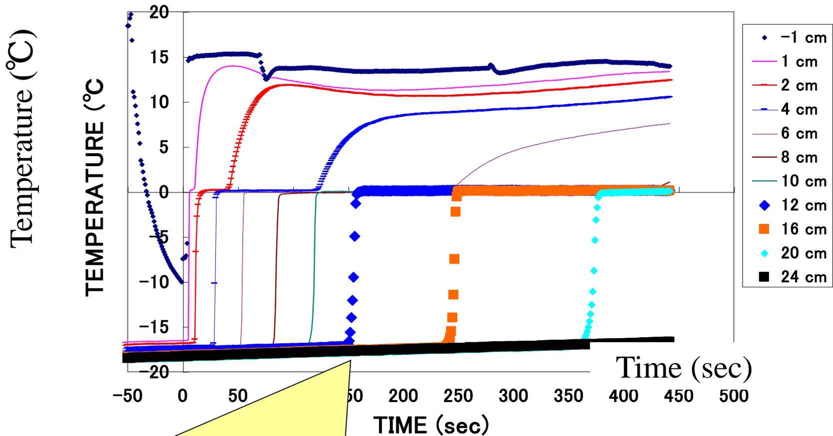
**Temperature increases abruptly to 0 °C when infiltration front reaches and keeps 0 °C for a while, then increases slowly.**
