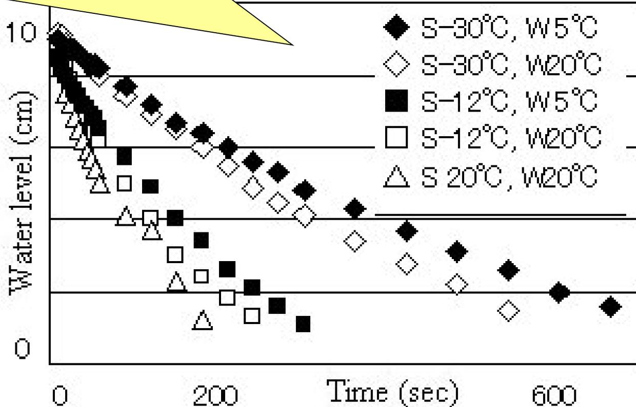
• Fig. 3 Changes in water level as a function of time during infiltration into dry sand columns.
