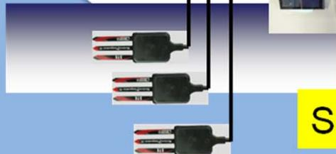
(Soil sensor : Soil moisture, temperature, electrical conductivity...)
