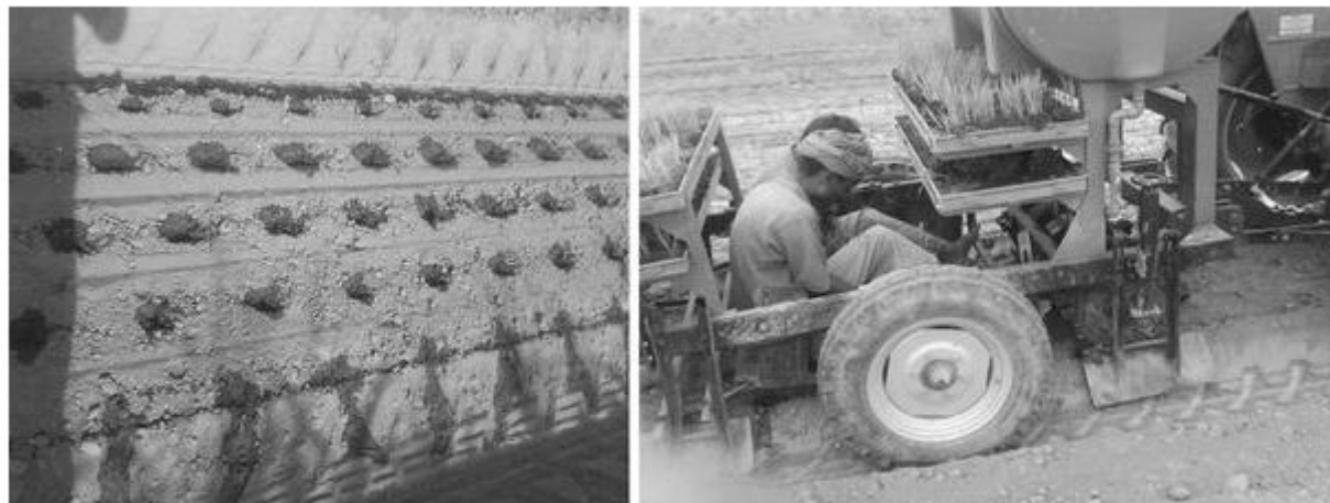
Fig. 1 Transplanting 10-day-old seedlings into a dry soil; note water tank above the supply of young seedlings
