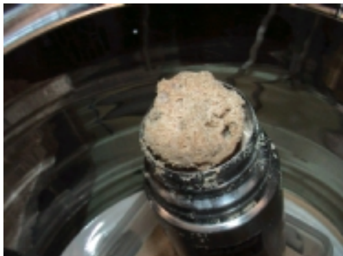
Fig.2 Frozen wet-sand in the chamber under vacuum
