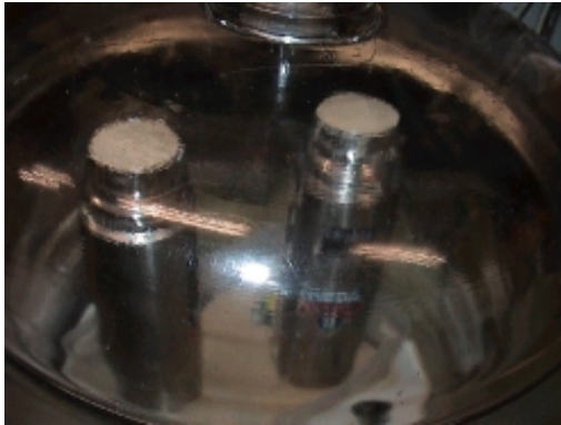
Fig.1 Sand columns in the chamber under vacuum
