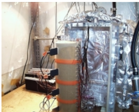
Fig.3 Sand column inserted sensors for the measurement of moisture content and temperature.
