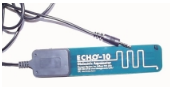
Fig.2 Soil moisture sensor (ECH 2 O-10) improved for this study.
