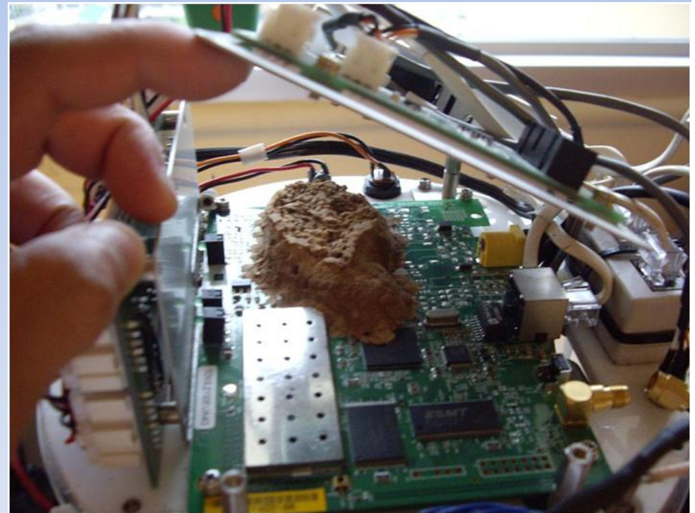
Insect nest built on CPU board of FS
