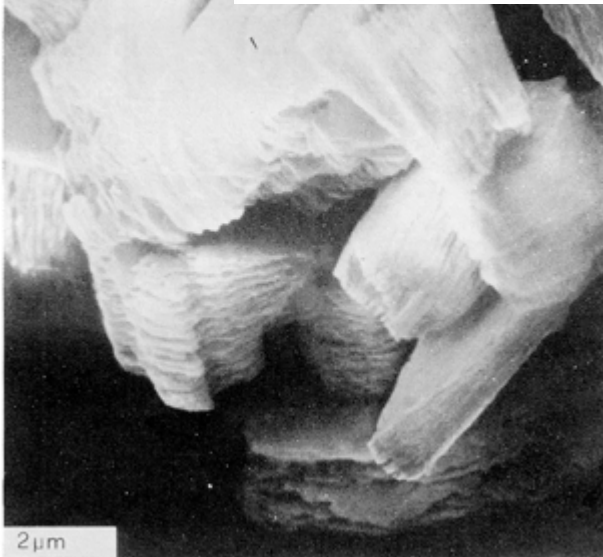
PLATE 2 Scanning electron micrograph of 8-5 μm size fraction of Georgia kaolin. This fraction contains well developed 'books' of platy kaolinite clusters (Lombardi et al. 1987)
