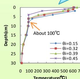
Fig.7 Temperature profile (Andisol  $t=6$  hrs)
