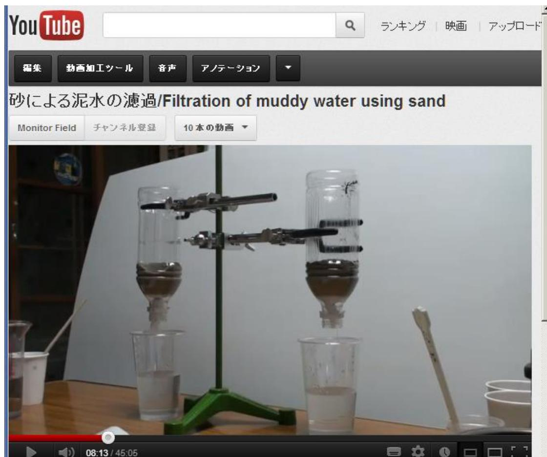
Fresh water comes out when muddy water is poured in the sand. When this operation is repeated, fresh water becomes slow to come out. Clay particles with radioactive cesium are also trapped in the sand by this principle.
