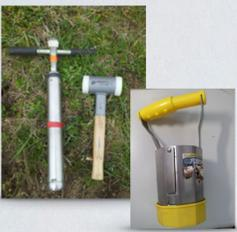
Soil samples were taken in agricultural field to analyze radiocaesium concentration every 1cm by Ge semiconductor detector. Also, the vertical distribution of radioactivity in soil was measured by the in-situ device.
