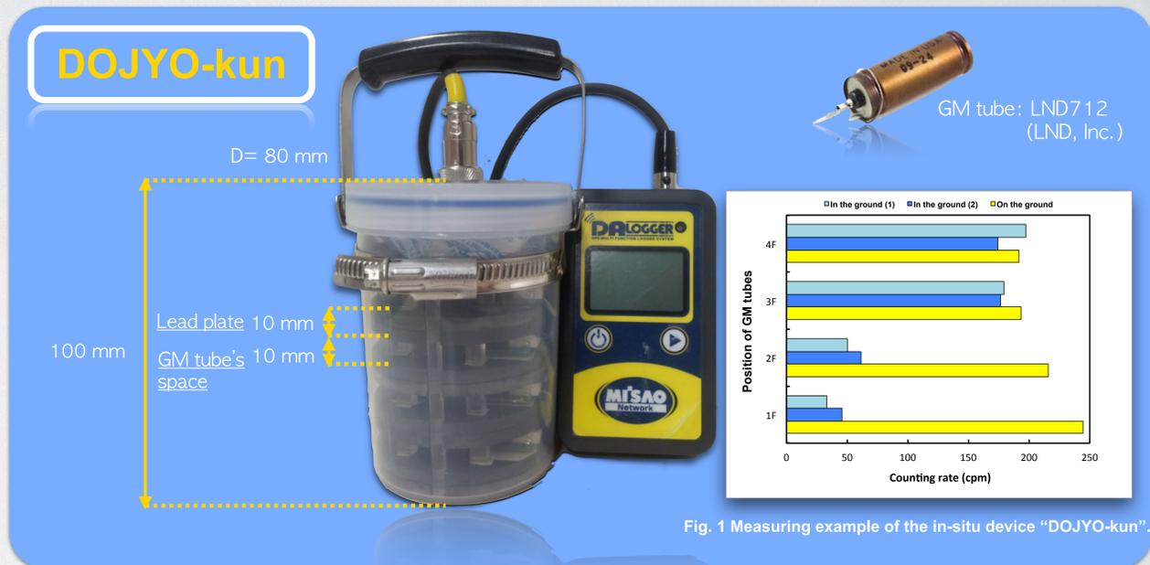
Fig. 1 Measuring example of the in-situ device "DOJYO-kun".
