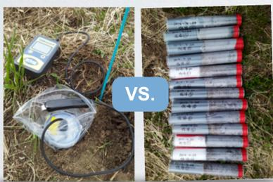
Radiocaesium concentration with the in-situ device was compared to that of soil samples taken.
